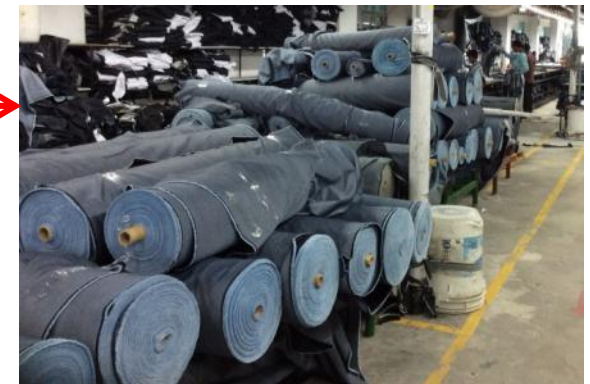
Uncontrolled stacking of materials.
