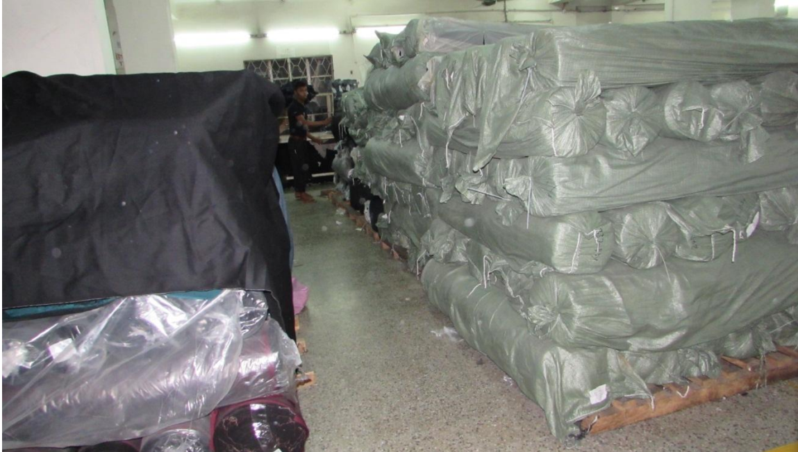
Excessive Storage Height of Fabric on Level 2
