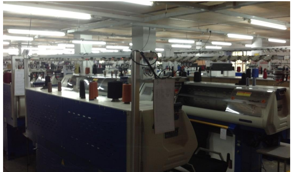
Jacquard machines at 2 nd Floor level
