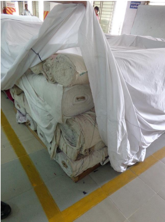
Storage of yarn rolls on the third floor slab. No loading plan visible.
