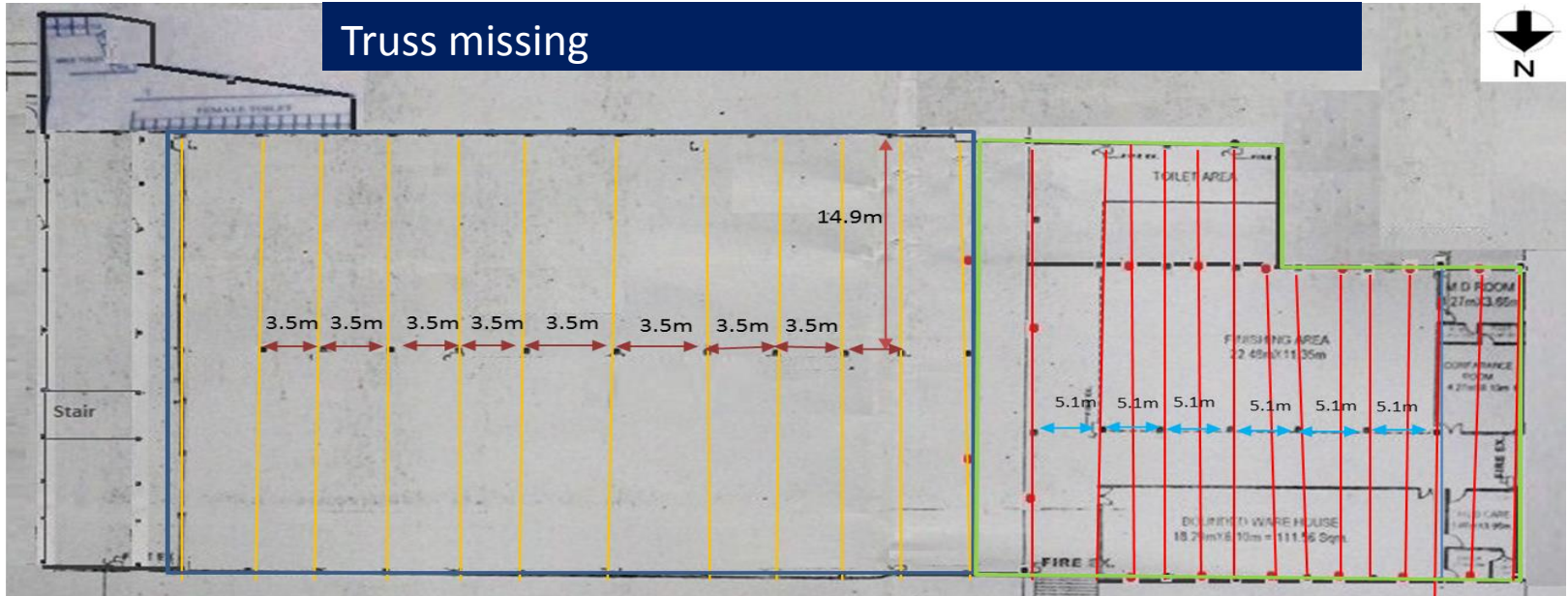
Column and steel truss layout plan
