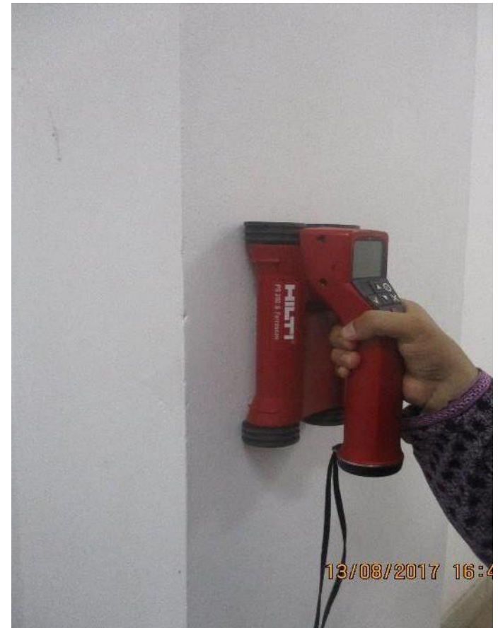
Rebar Scanning of column
