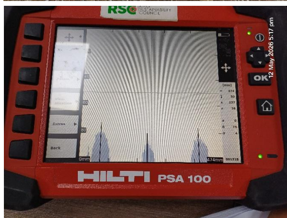
(Scan of RC2 Column short face, at Grid Point J8 of 4 th floor)
