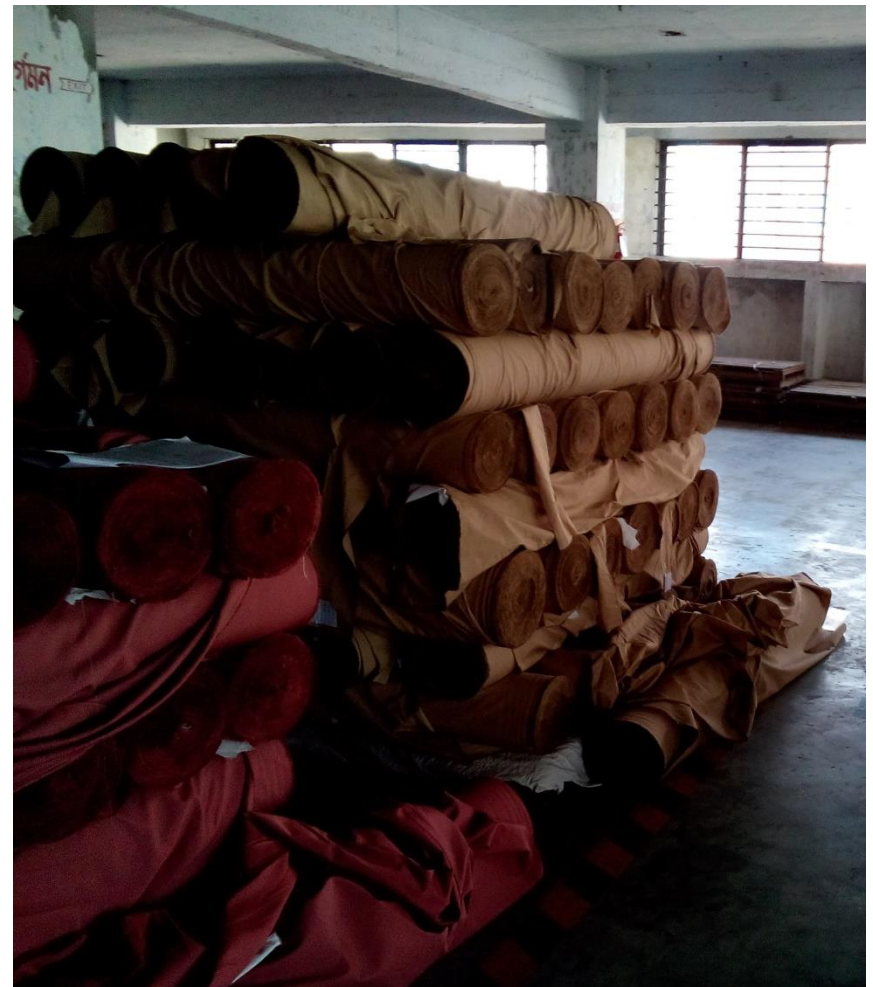
Uncontrolled stacking of fabric roll
