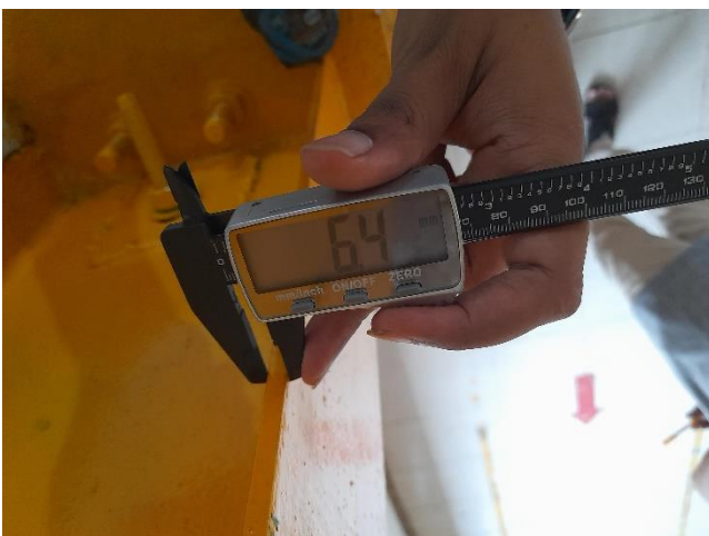
RB1 was measured as 350x475 mm which was shown as 300x475 mm in the drawing
