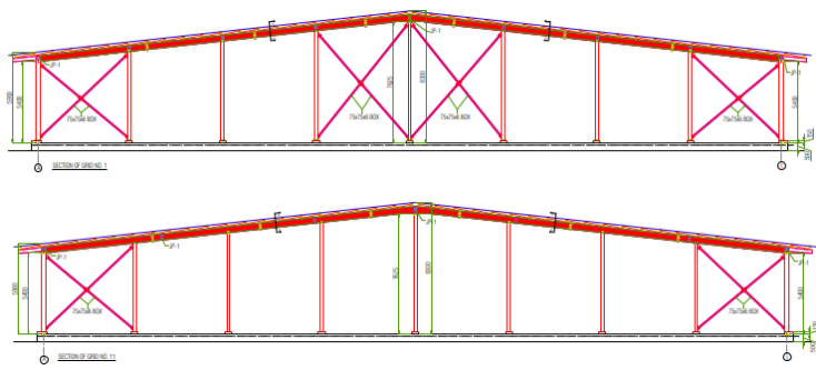
Proposed wall bracing and rafter retrofitting
