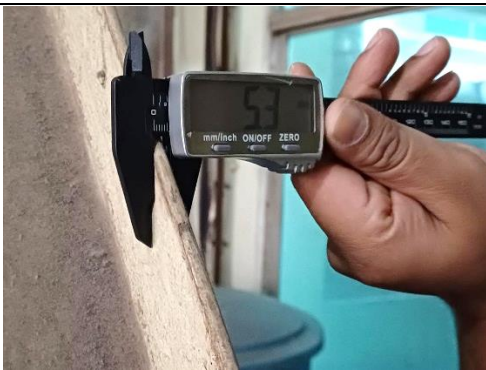
The thickness of wall bracing was found 5.3 mm instead of 6 mm
