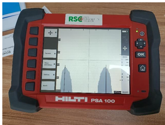
Number of rebar by ferro scan
