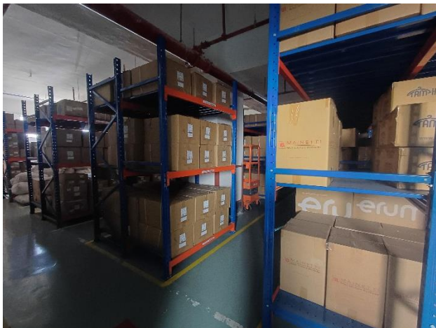
Unbraced racks on the floor
