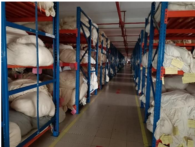
Unbraced racks on floor
