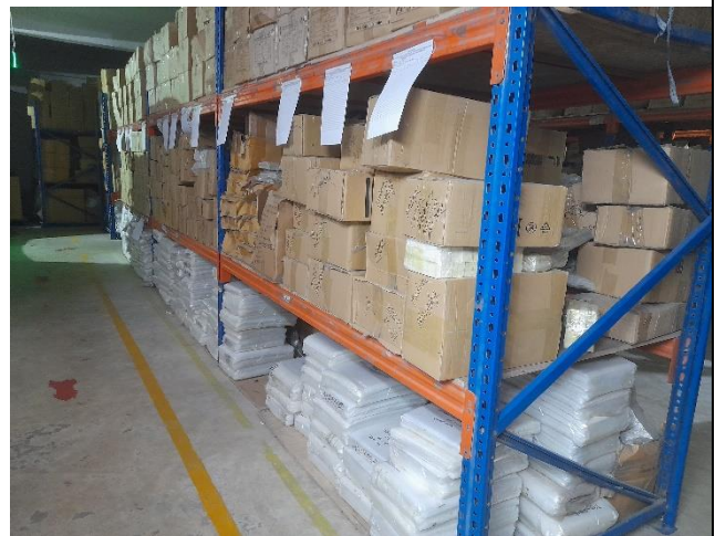
Unbraced storage racks on floors
