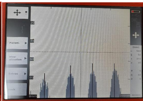
Ferro-scanning at 5 th floor
