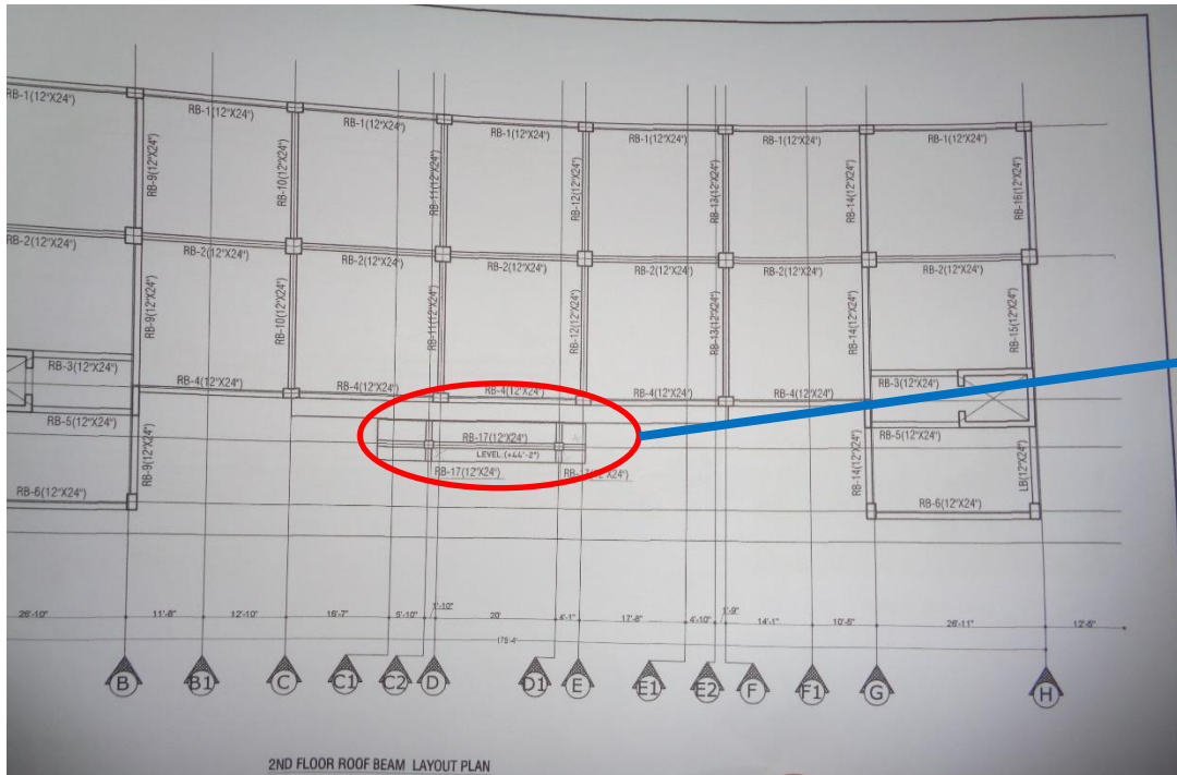
Marked beams layout not matched with on-site condition
