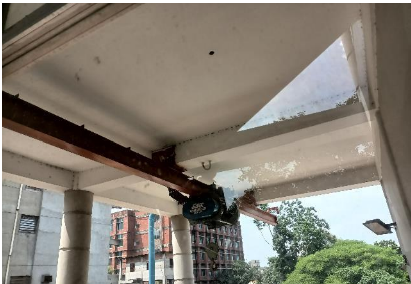
Overhang crane suspended from beam
