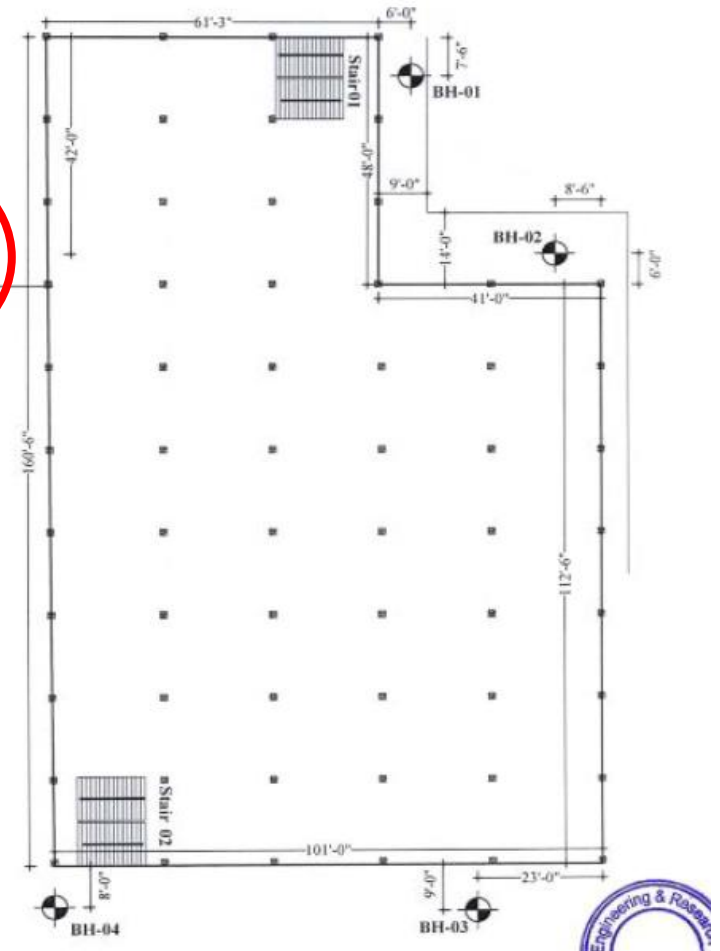
Borehole layout of Dry Process Building
