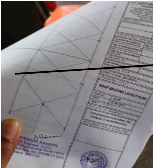
Bracings were connected apart from column-rafter joint
