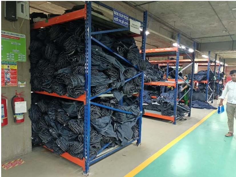
Storage racks not anchored or braced
