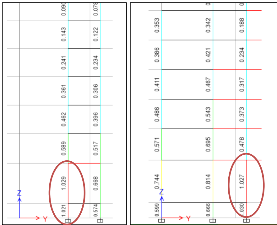
Overstress column in FEA model
