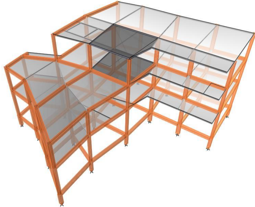
Irregular building shape and flat slab system
