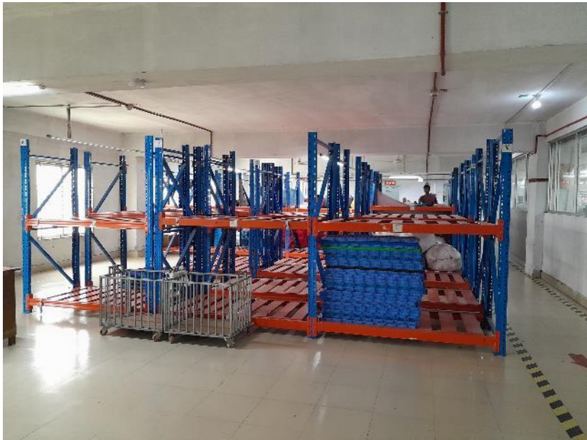
Lack of anchorage/brace of storage racks
