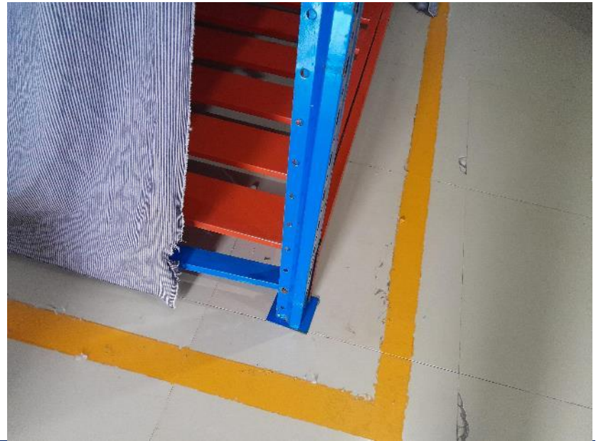
Lack of anchorage/brace of storage racks
