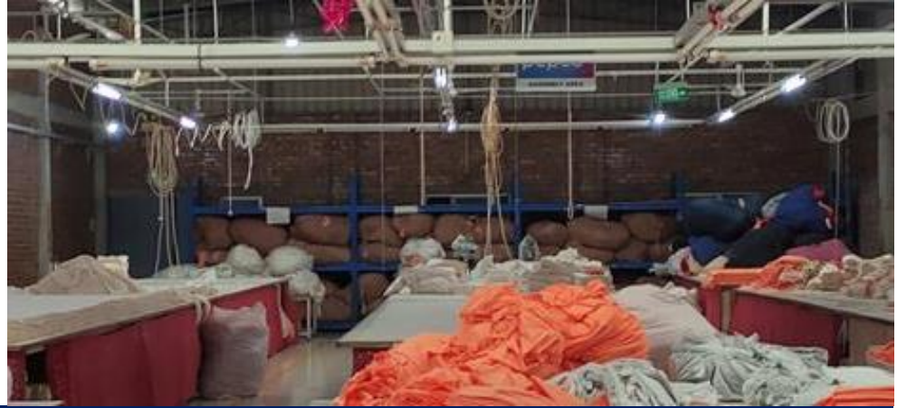
Unbraced storage rack
