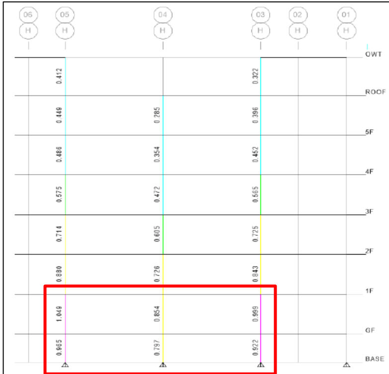
Figure 3.1.8: PMM ratio of Column in Grid H'
