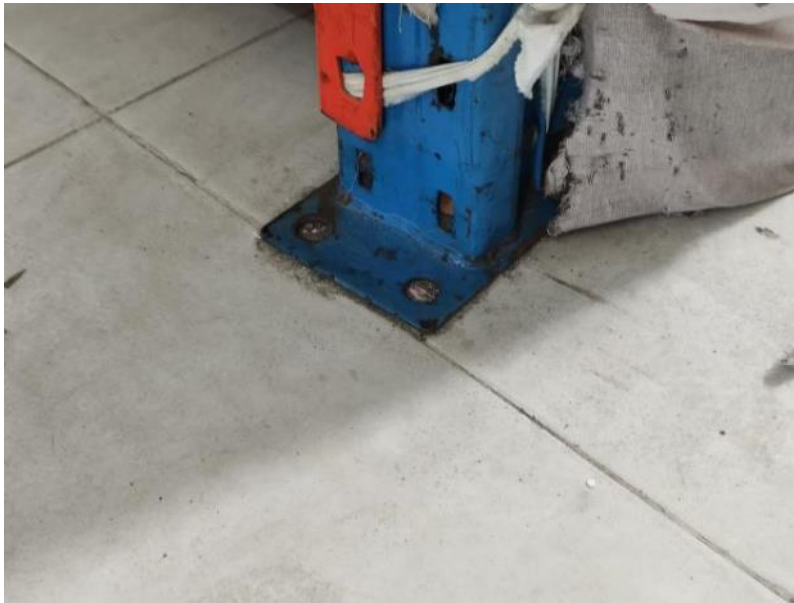
Lack of anchorage of storage rack
