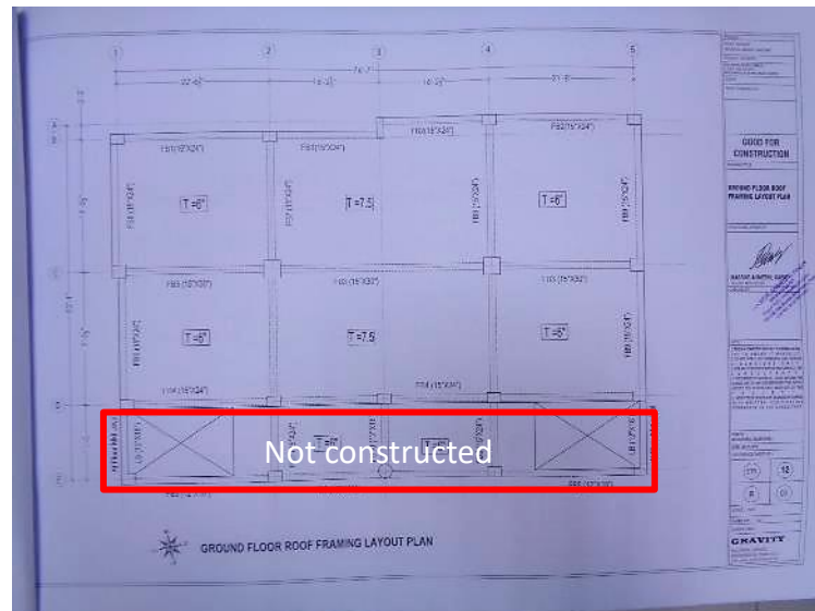
Ground floor roof beam layout
