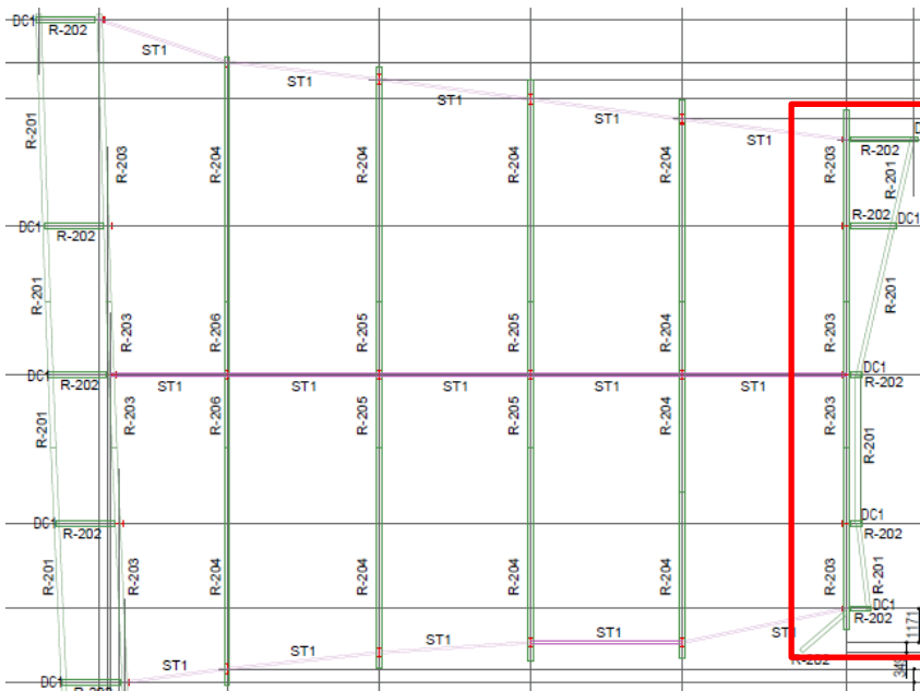
Rafter Layout: Irregular column layout and beam arrangement
