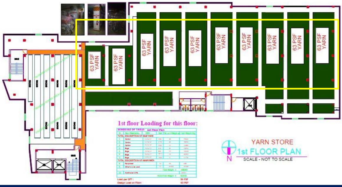
Load plan for 1st floor (Yarn store-3KPa)
