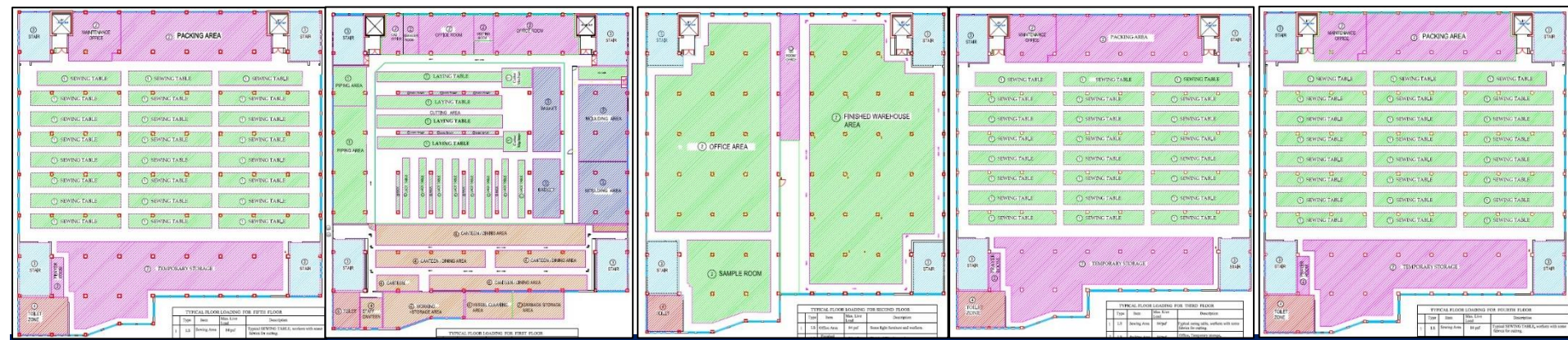
Load plan for 1 st to 5 th floor. - Floor loading has been shown (84 psf) 4 kPa.
