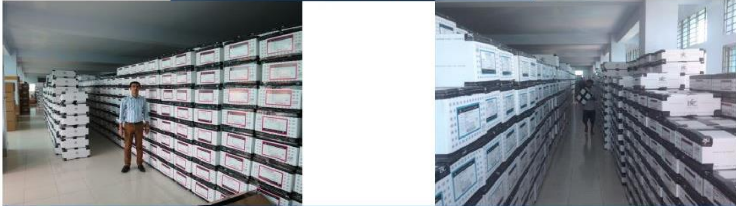
Finished Goods stored throughout floor area. Average the loading on that floor was 2.5Kpa
