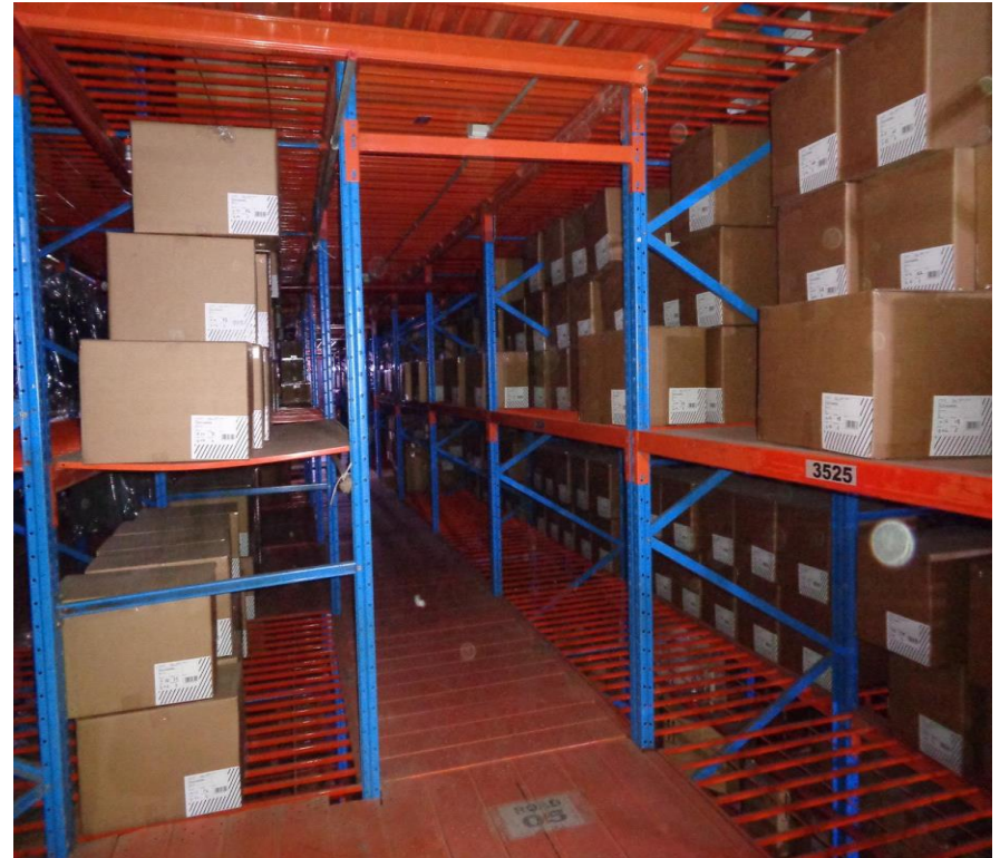
Storage load resting on multi storied steel rack
