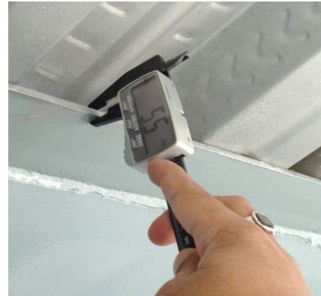
Flange thickness found 5mm
