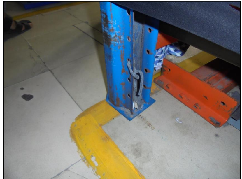
No anchoring with floor
