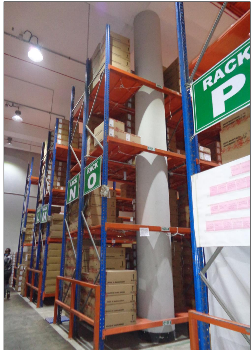
Storage load resting on multi storied steel rack
