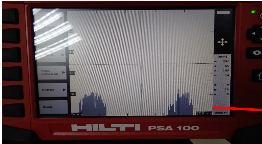
Ferro-scan shows 2-rebar along short face instead of 3-rebar (C-5)
