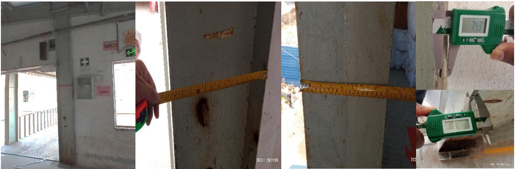
Miss match in column at 1 st floor (SC-3A found 390x200x7 instead of 400x230x8)
