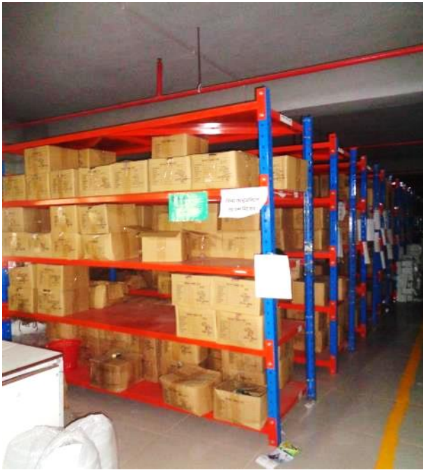
Storage rack without bracing and not anchored
