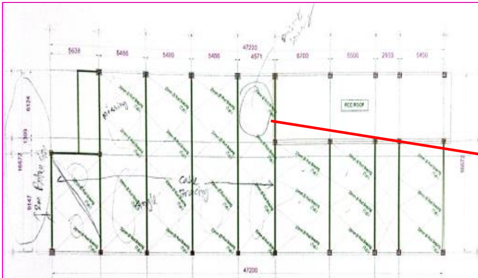
Missing bracing at roof
