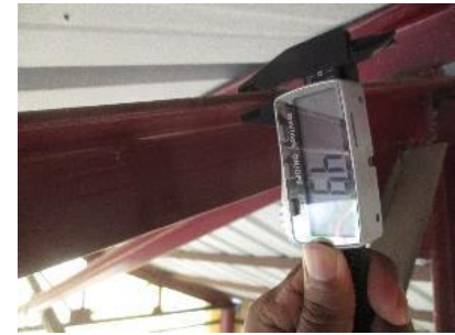
Top & Bottom Chord and bracing thickness 5mm instead 6mm
