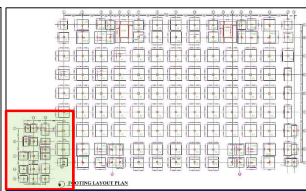
Foundation layout plan- marked portion toilet block
