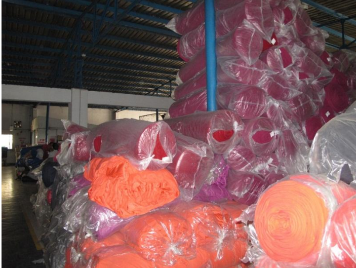
Uncontrolled heavy storage on ground and 4 th floor. (GF not a problem).
