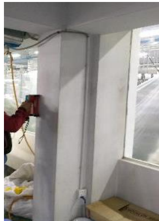
Additional column confirmed by scanning
