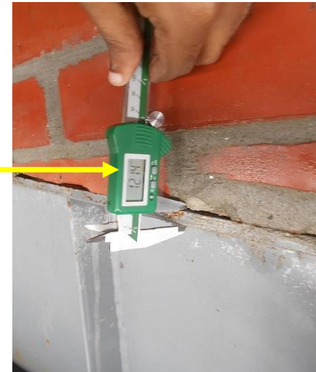
12 mm thick flange instead of 14 mm
