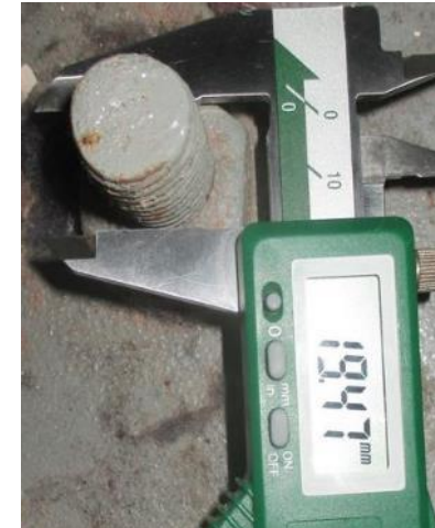
Anchor bolts were 20 mm instead of 25 mm.
