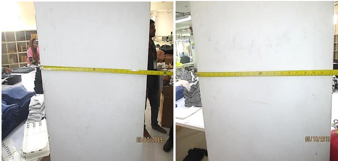
Size of C10 column was found 500mmX500 mm
