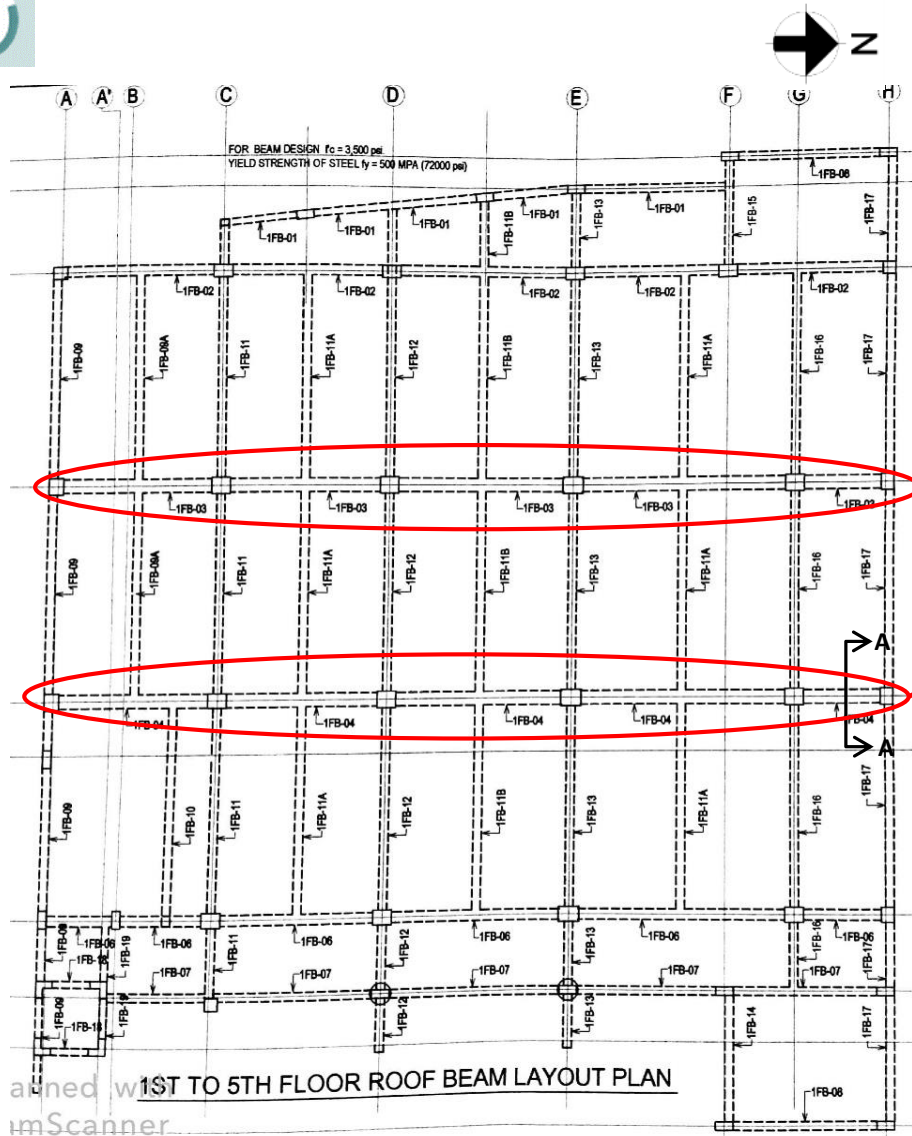
1 st to 5 th floor roof beam layout
