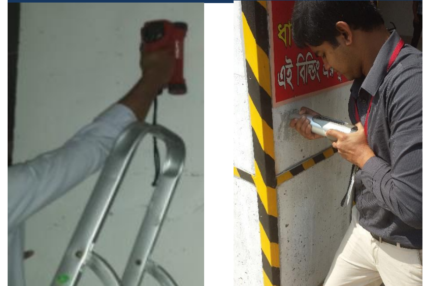
Records of Ferro scanning & Schmidt Hammer tests
