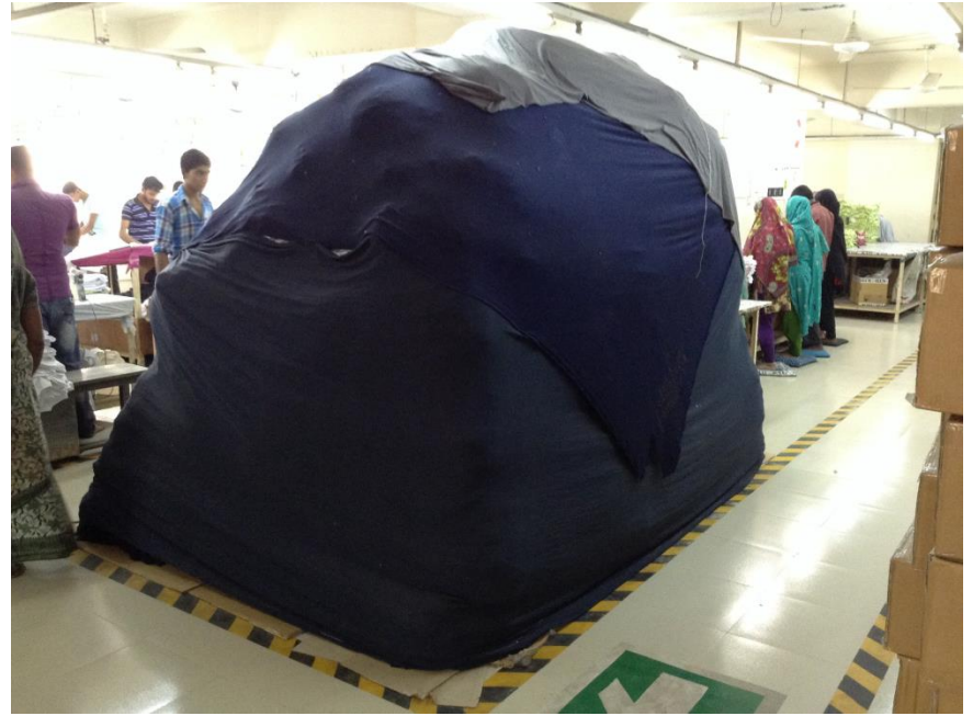
Heavy loads, approximately 5kPa to 8kPa observed on 1 st floor
