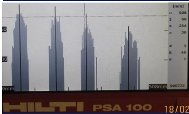
Rebar in long face
